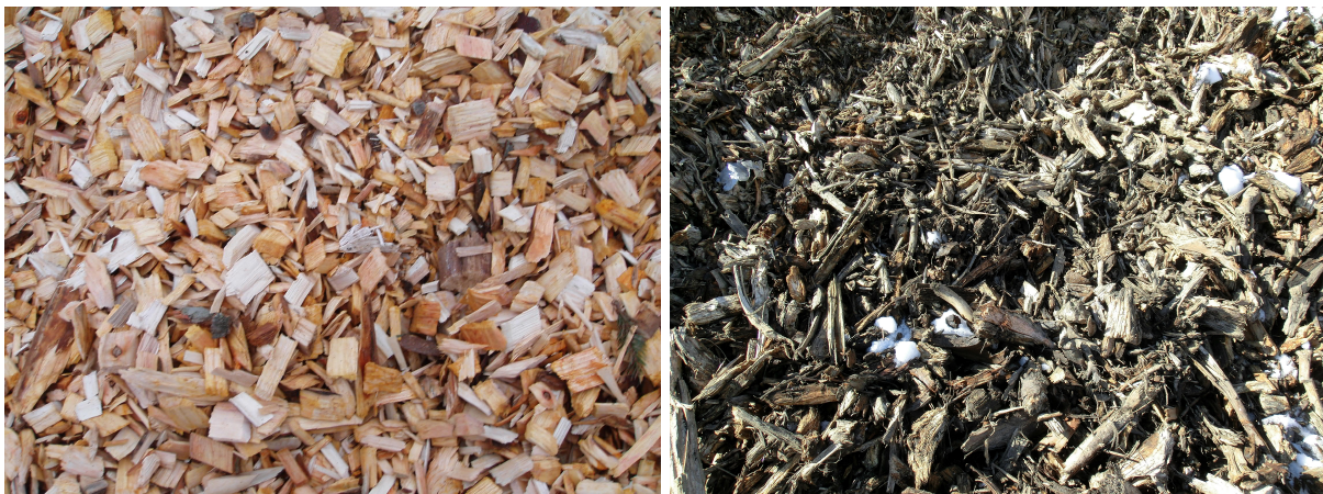
Figure 3. The result of two different comminution techniques: chipped roundwood (left) and grinded stump biomass (right). (Photo: Eriksson, Anders)
