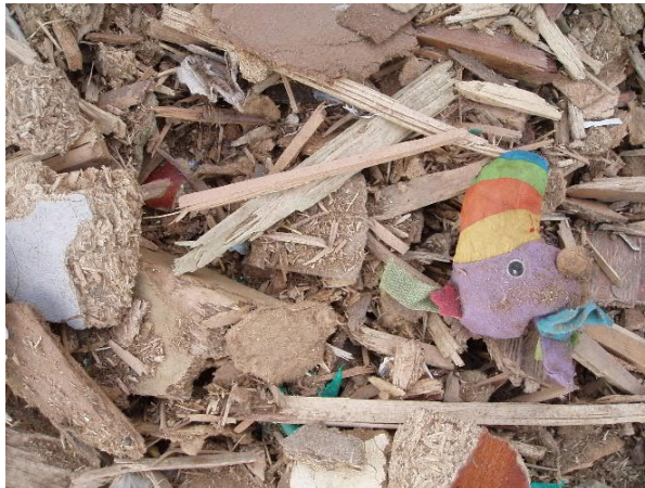
Figure 8. Waste wood chips at a Swedish district heating plant. (Photo: Eriksson, Anders)
