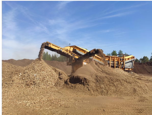
Figure 2. Quality enhancement by separation through screening of logging residue chips into a coarser accept fraction and a finer reject fraction. (Photo: Eriksson, Anders)
